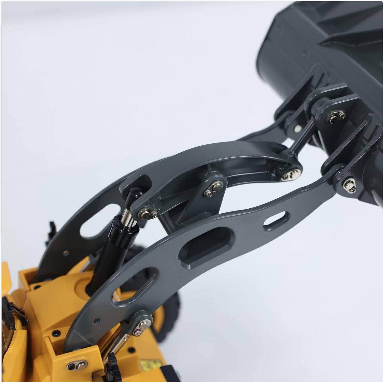
Image: Detailed view of the loader's bucket and its hydraulic-like lifting arms, showcasing the robust metal construction and pivot points.
