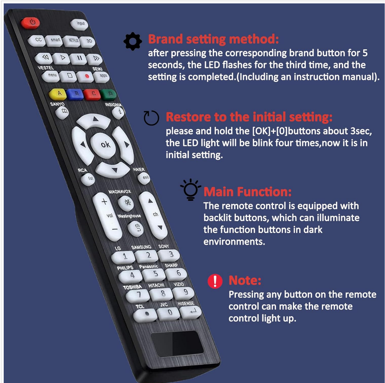
Image 6: A visual guide detailing the brand setting method, showing the remote and instructions to press and hold the corresponding brand button until the TV turns off.
