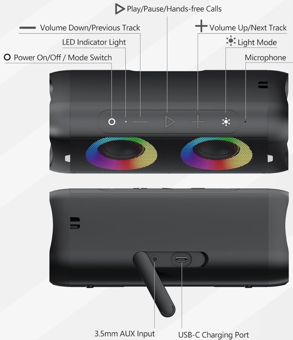
Image 6: Detailed diagram of the speaker's top panel buttons and rear ports for operational guidance.
