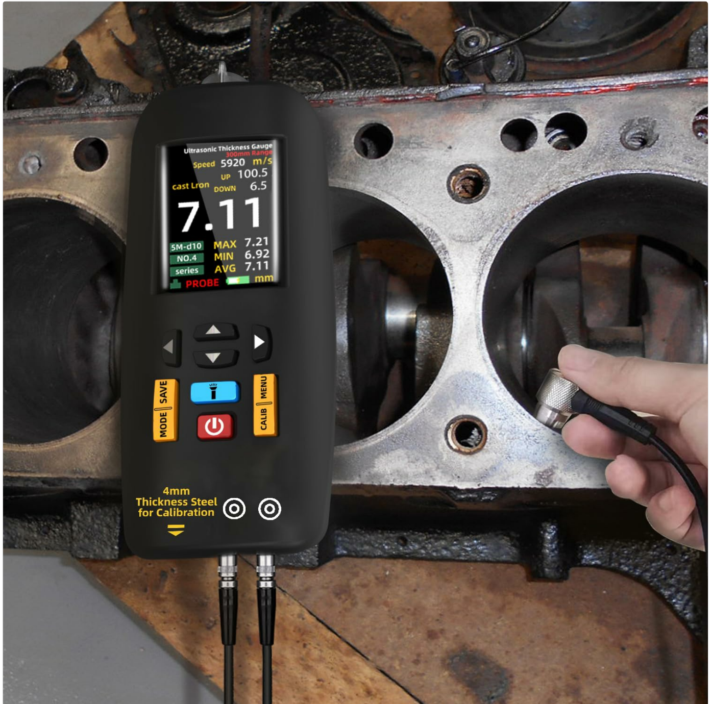
Image: The BSIDE Ultrasonic Thickness Gauge in active use, with its probe placed on a metal engine block to measure its thickness, demonstrating a typical application.
