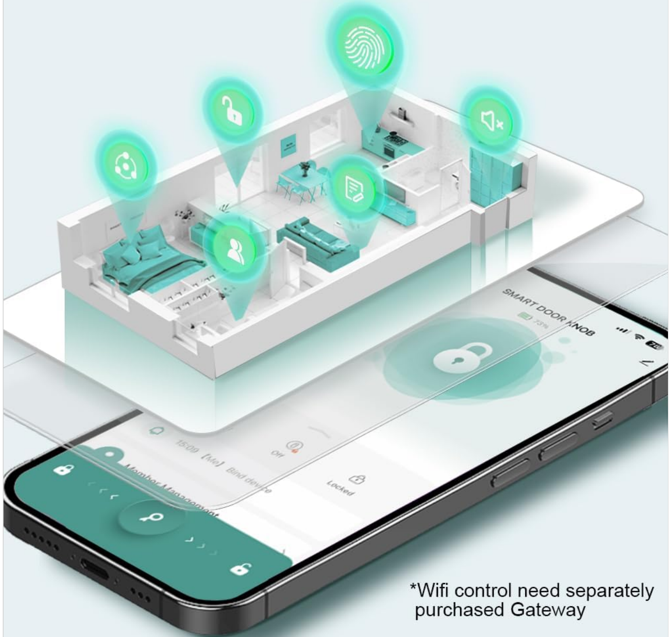
Figure 5: The smartphone app provides essential features including passage mode, auto-lock, fingerprint setting, user management, record checking, and silent mode.
