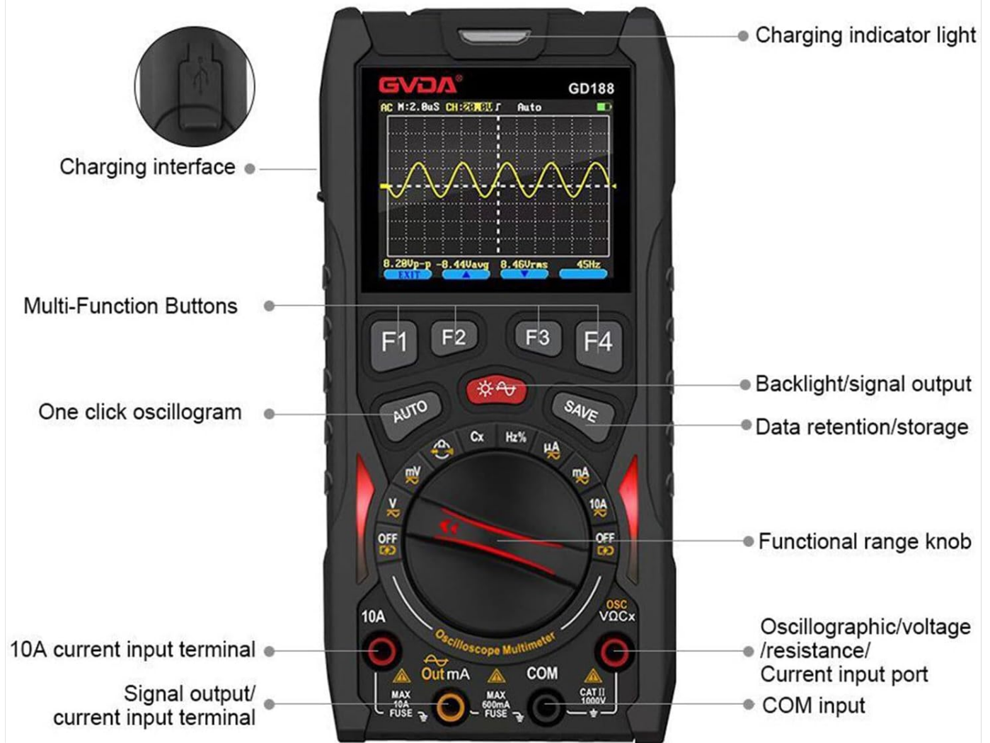
Figure 2: Labeled diagram of the GD188 showing key components like the charging interface, multi-function buttons, display, and input terminals.
