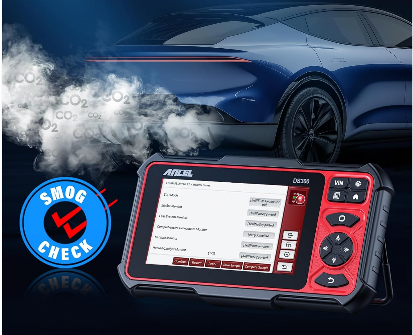
Figure 4.7: Are You Inspection-Ready? This image displays the DS300 screen showing the status of emission monitors for an I/M readiness check, indicating whether the vehicle is ready for a smog inspection.
