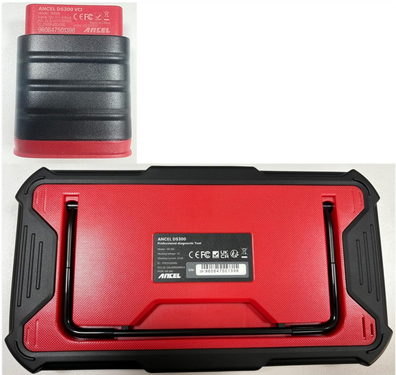
Figure 2.1: Rear view of the DS300 main unit and the Bluetooth VCI module. This image shows the back of the DS300 scanner, highlighting its integrated stand, and the separate Bluetooth VCI module.
