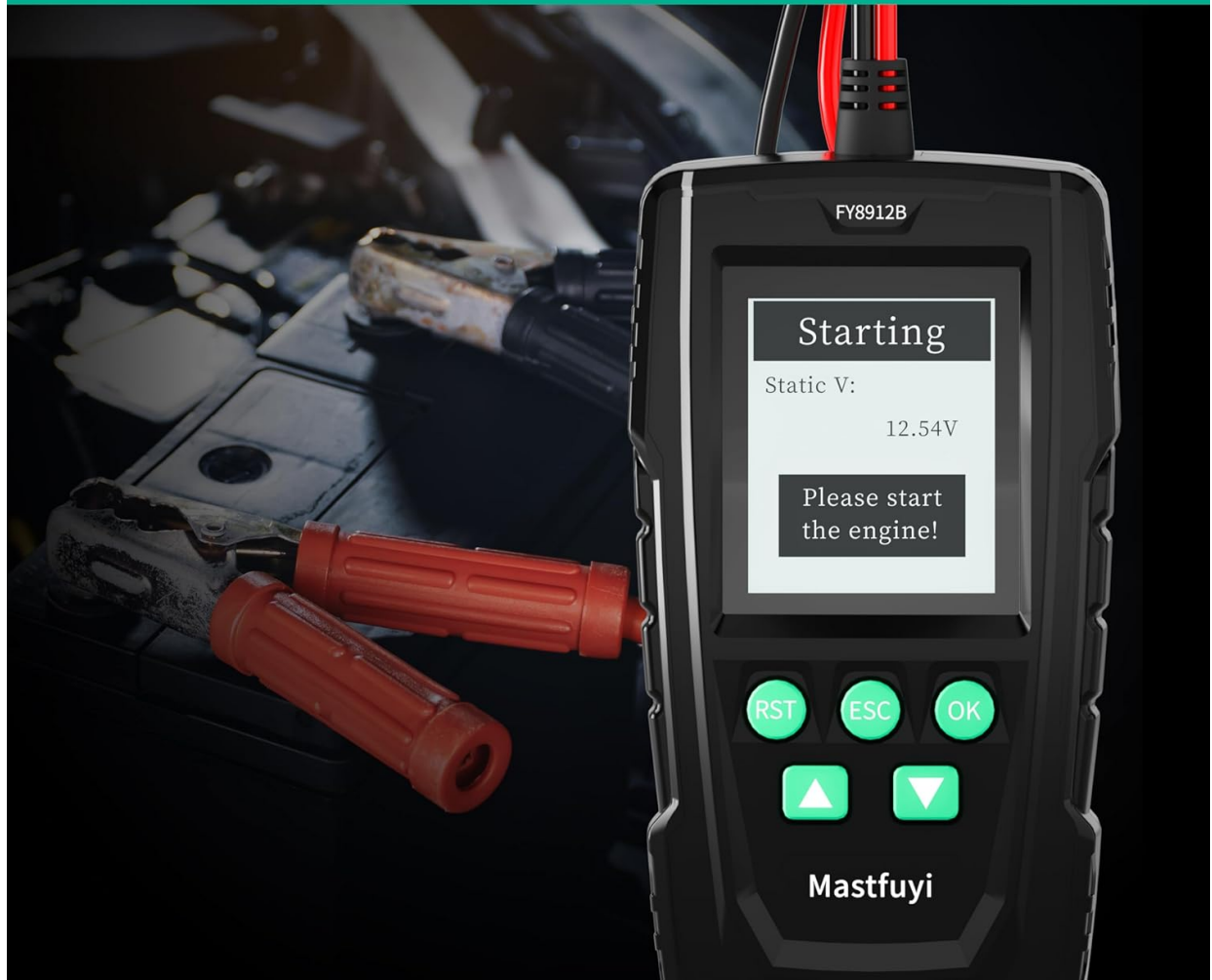
Image 6: The tester's screen during a 'Cranking/Starter Test', prompting the user to 'Please start the engine!' and showing a static voltage of 12.54V.
