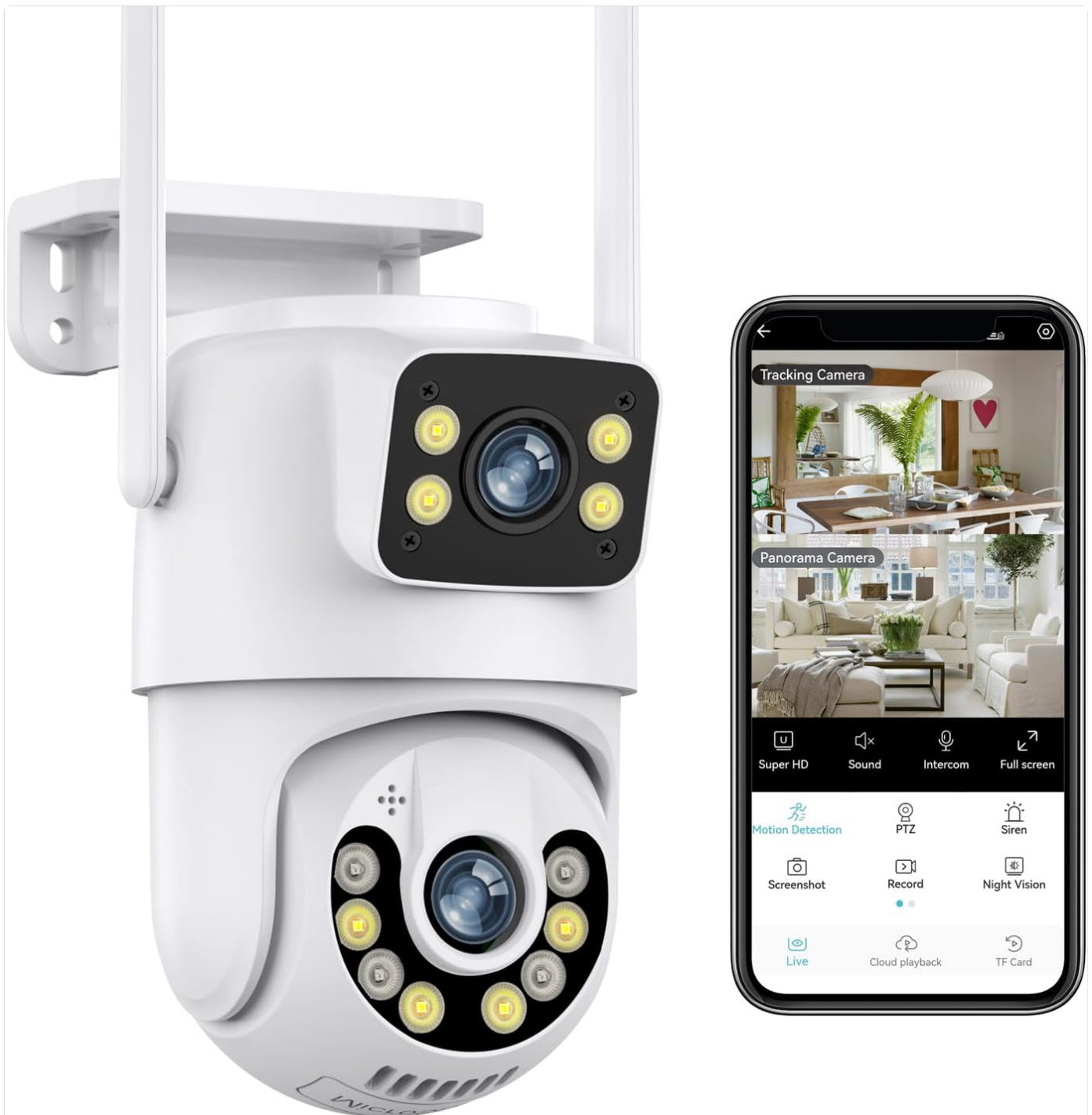
Image: The Dosilkc 1080P PTZ Outdoor Security Camera, showcasing its dual lens design and two antennas, alongside a smartphone displaying the camera's app interface with live views.
