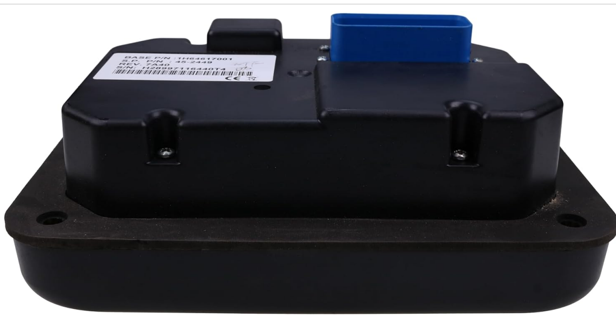
Figure 3: Rear view of the LSSOCH Smart Reefer SR4 HMI Controller, showing the product label with part numbers and the blue multi-pin connector.
