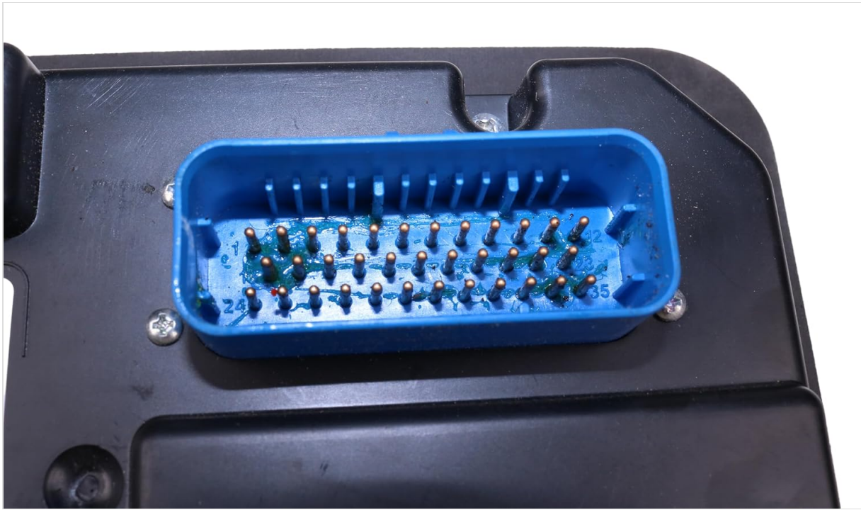
Figure 4: Close-up view of the blue multi-pin connector on the rear of the LSSOCH Smart Reefer SR4 HMI Controller, detailing the pin configuration.
