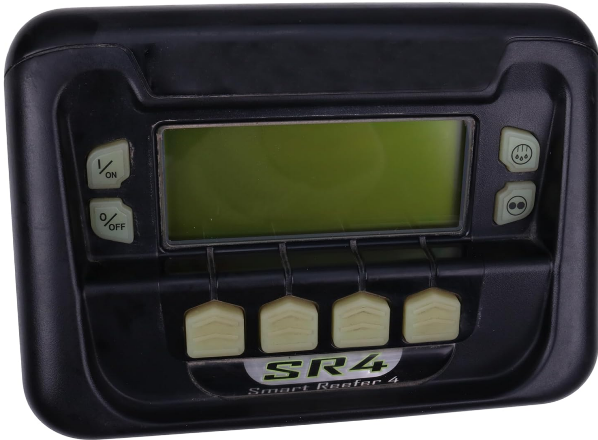
Figure 2: Front view of the LSSOCH Smart Reefer SR4 HMI Controller, highlighting the central display and the arrangement of the power and function buttons.
