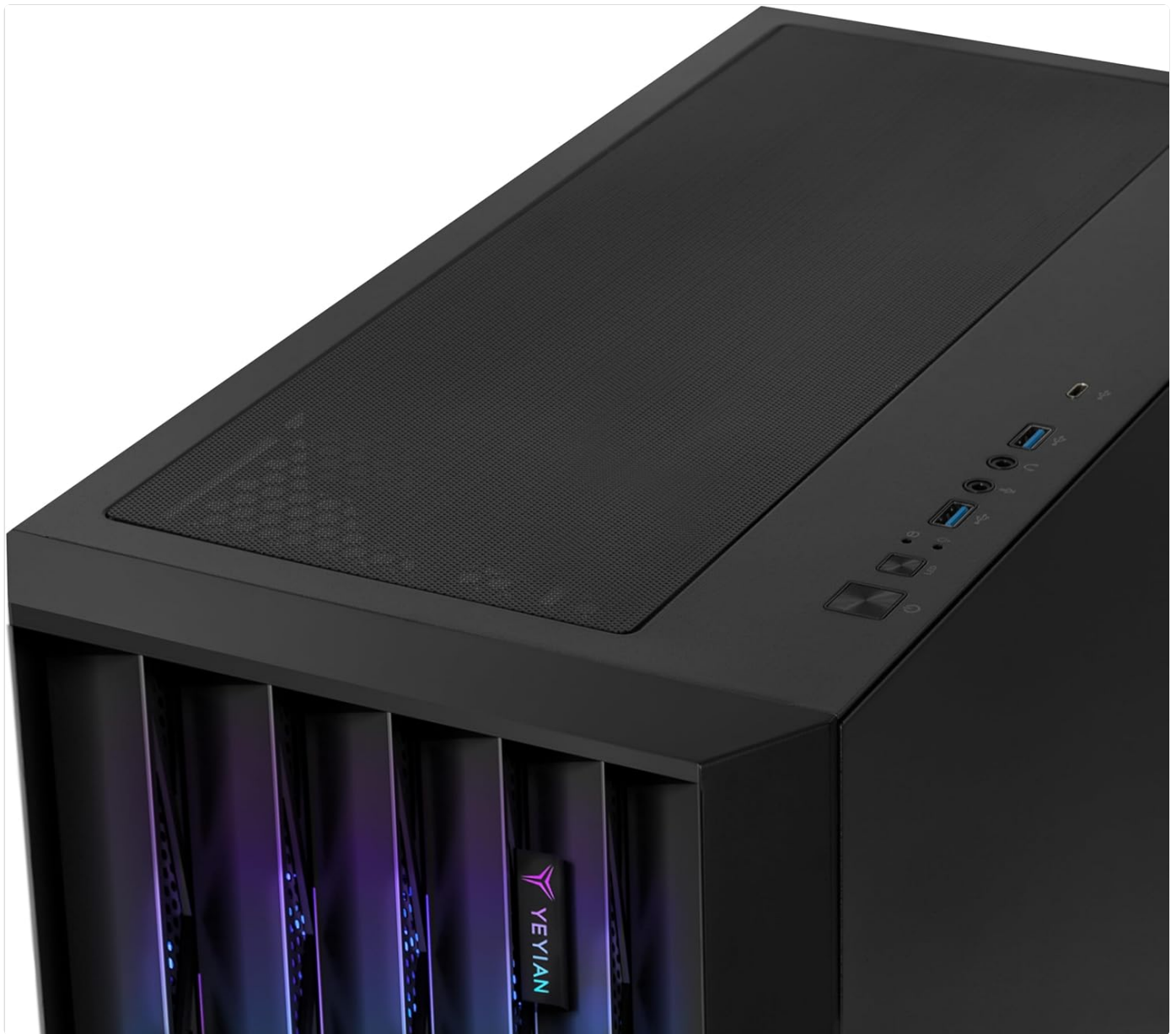
Figure 5: Top I/O panel with various ports and buttons.
