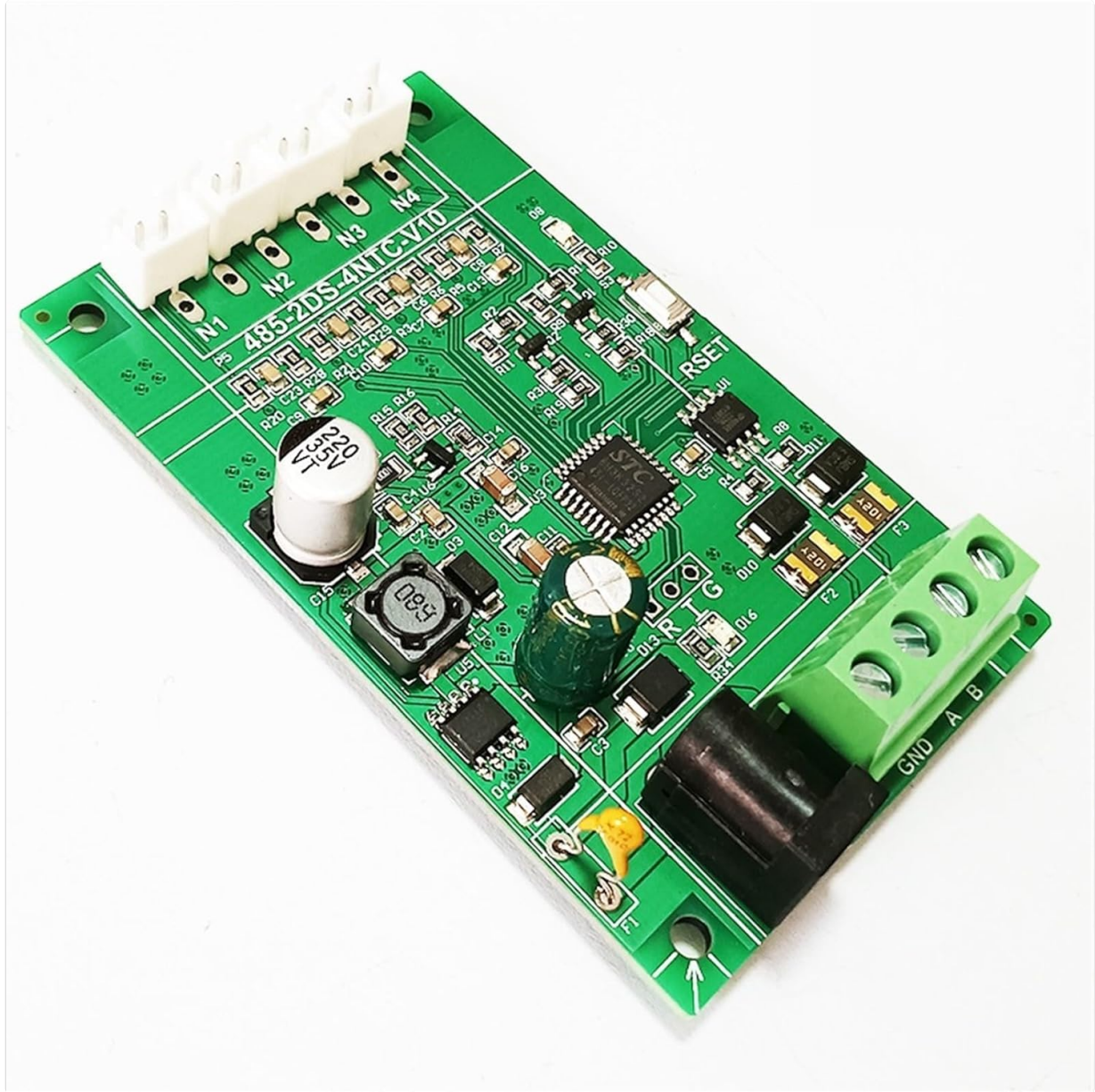
The bare circuit board of the CEMELI 4-Channel NTC Temperature Transmitter, highlighting the electronic components, NTC sensor input terminals (N1-N4), and the power/RS485 screw terminals.
