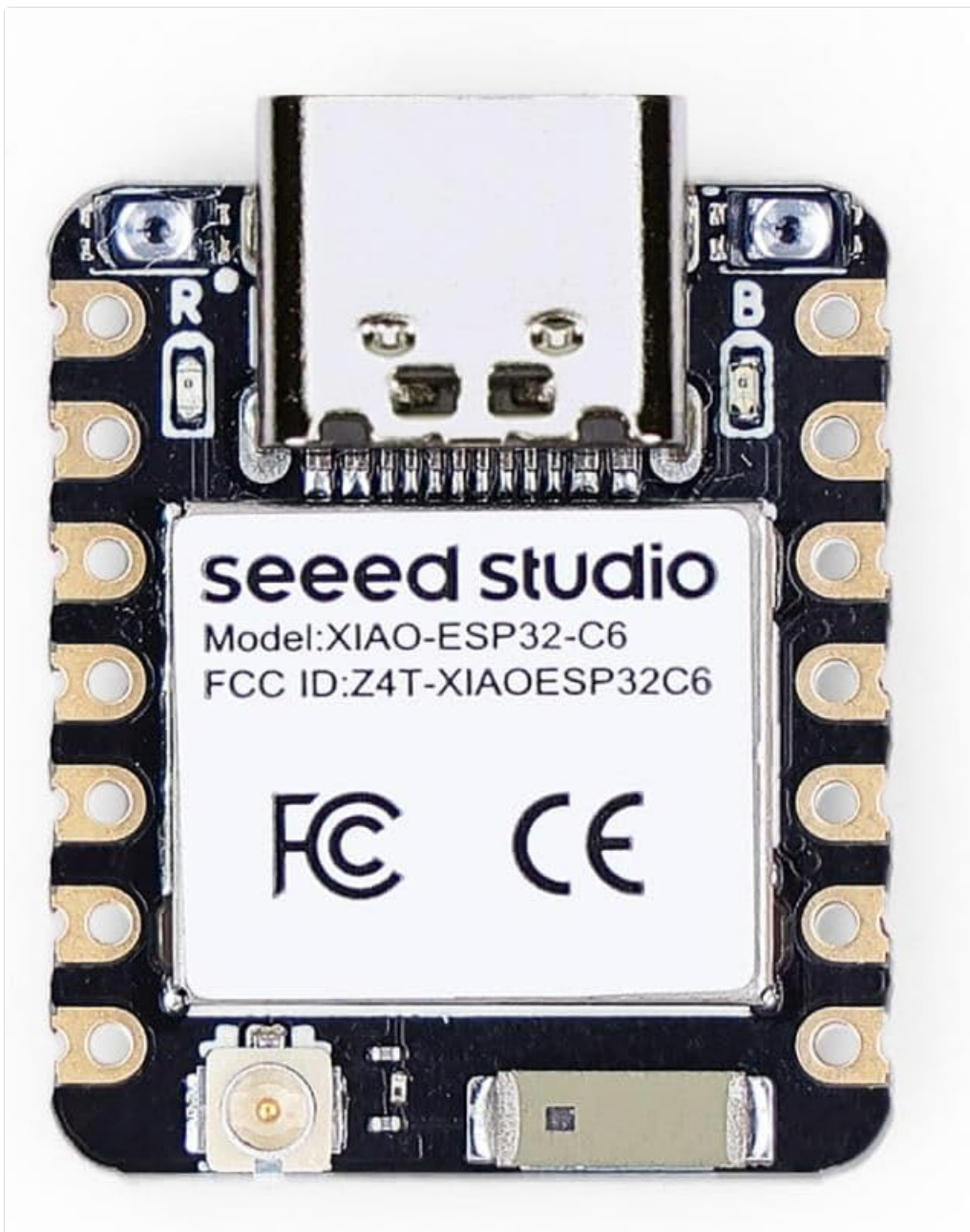
Image 1.1: Front view of the Seeed Studio XIAO ESP32C6 board, showing the USB-C port and main chip.
