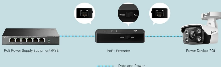
Figure 1: The TP-Link POE10E PoE+ Extender is designed to extend the range of a PoE network connection.
