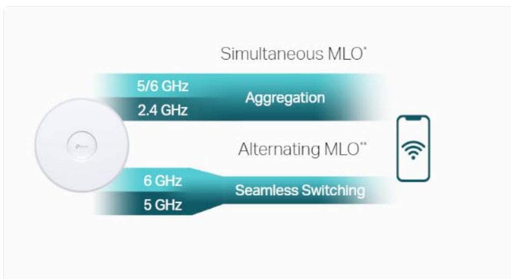
Figure 5.3: Explanation of Multi-Link Operation (MLO), demonstrating how the EAP772 can aggregate or seamlessly switch between different frequency bands for optimal performance.
