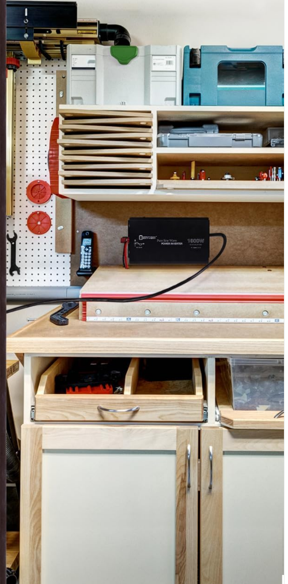
Image: The wired remote control displaying battery voltage, AC output voltage, power output, and various protection indicators. The inverter is visible in the background.
