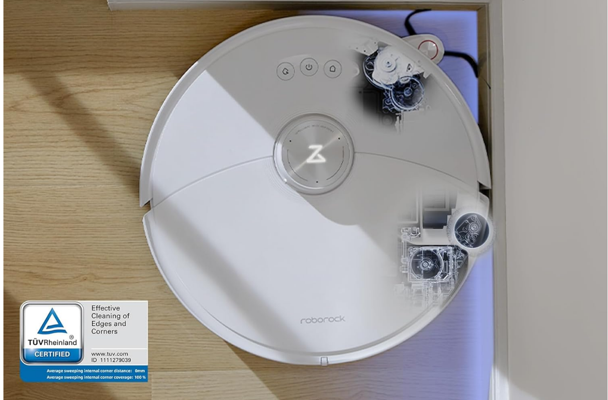
Image 3.2: The FlexiArm side brush extending to clean tight corners and edges.
