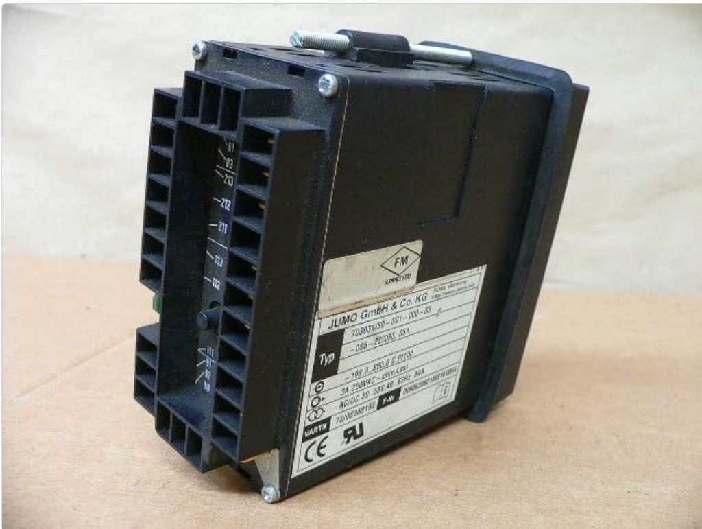
Figure 2: Close-up view of the product label on the Jumo Dtron 08.1 Temperature Controller, showing detailed specifications including model number, temperature range, and electrical ratings.
