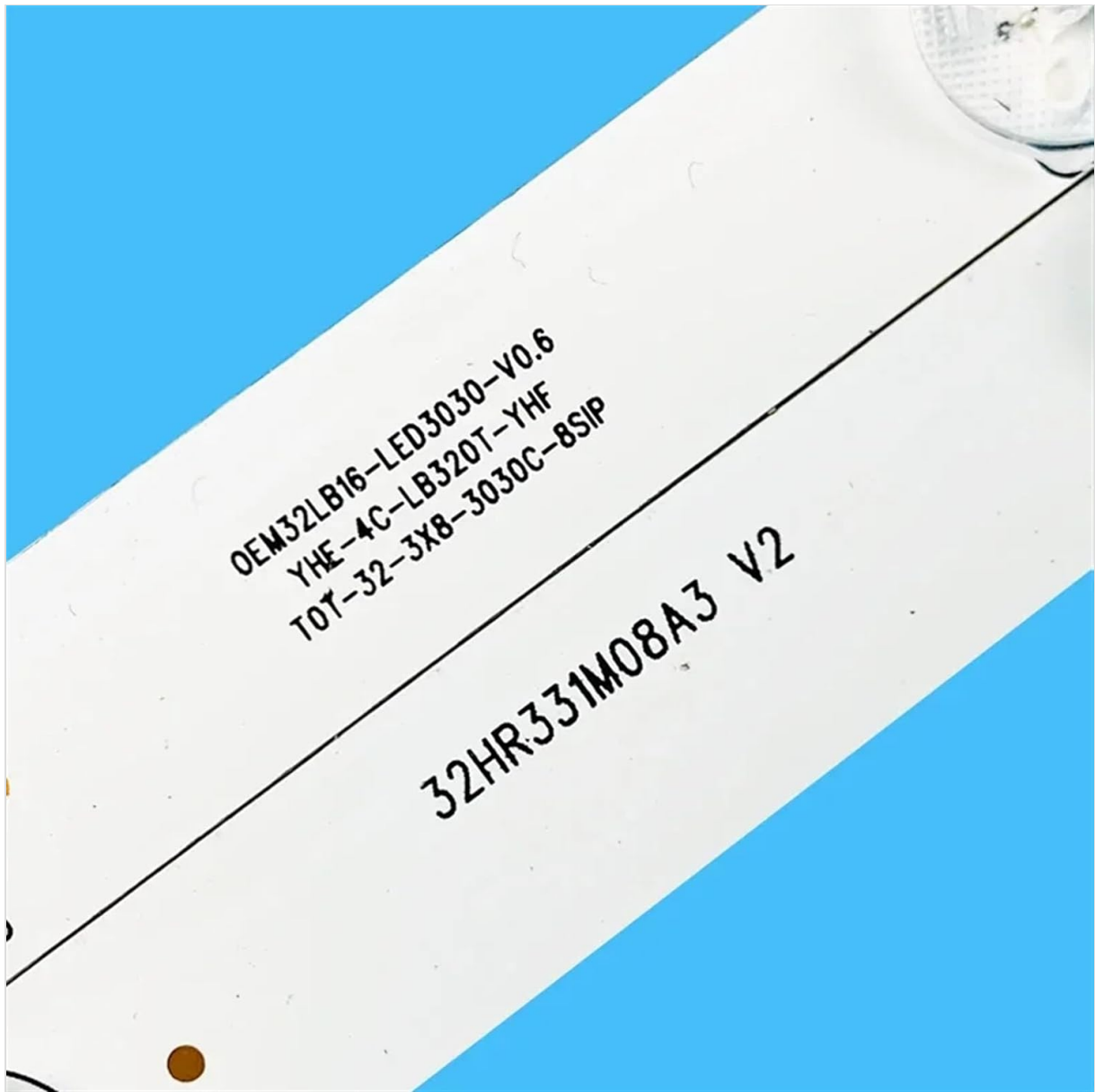
Another detailed view of the LED strip's identification markings, showing part numbers such as OEM32LB16-LED3030-V0.6 and 32HR331M08A3 V2. These markings assist in confirming the correct replacement part.
