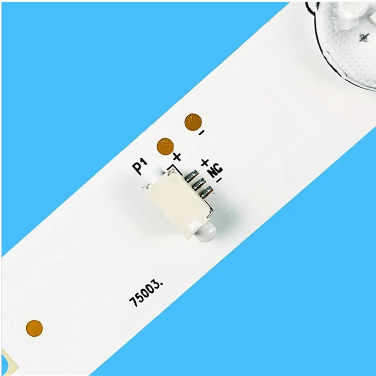
A close-up image of the electrical connector on the LED backlight strip, labeled P1, with positive (+), negative (-), and No Connection (NC) pins, along with the number 75003. This connector is used to supply power to the LED strip.
