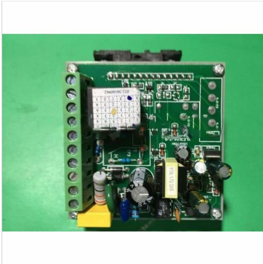
Image 4: A detailed view of the circuit board for the YLE-3000 YLE-3108 Temperature Driver, highlighting the terminal blocks for electrical connections.
