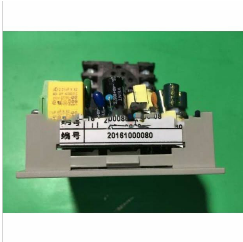
Image 3: A view of the internal components of the YLE-3000 YLE-3108 Temperature Driver, showing various electronic parts mounted on a circuit board.
