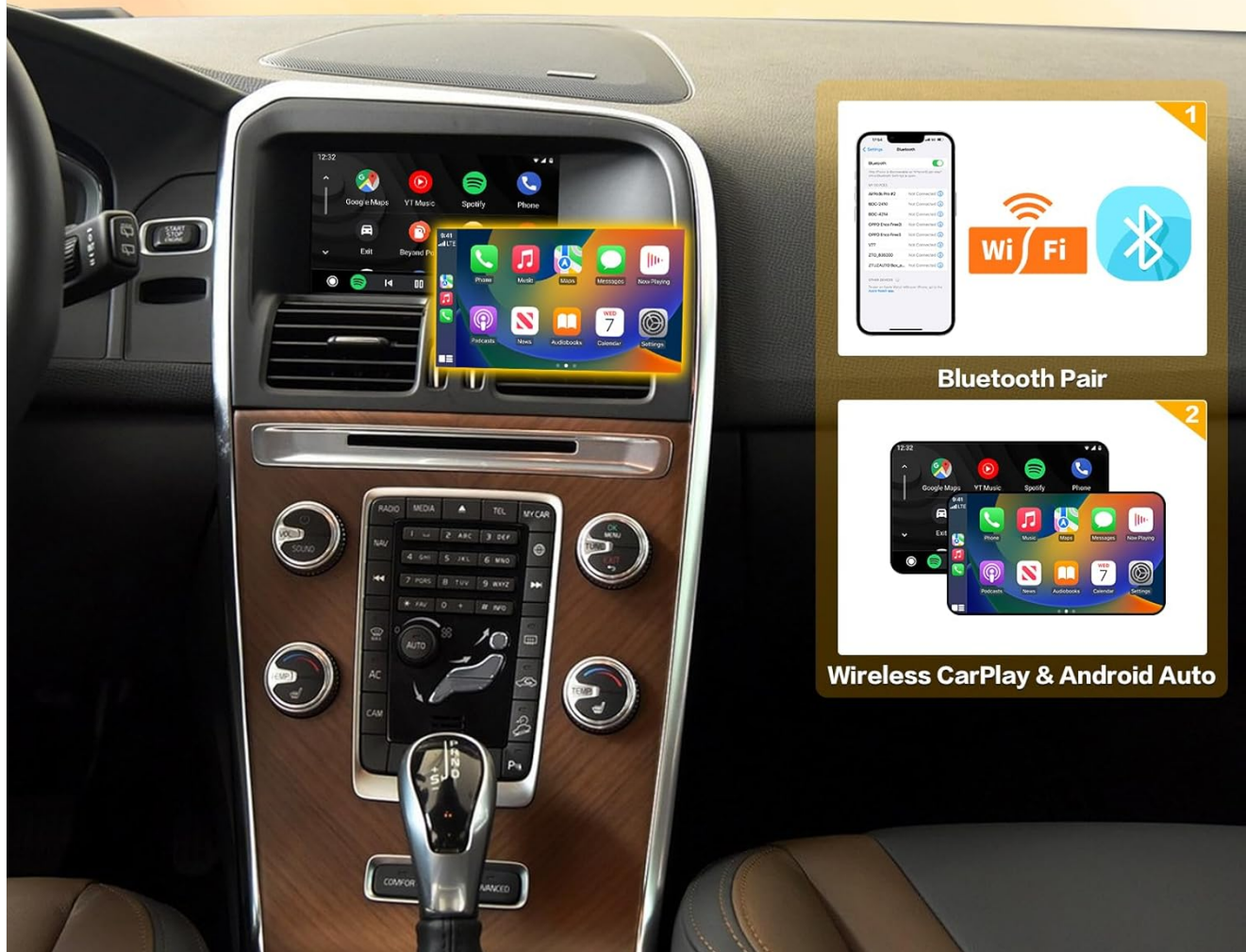
Image 5.2: Steps for establishing a wireless connection for CarPlay or Android Auto.
