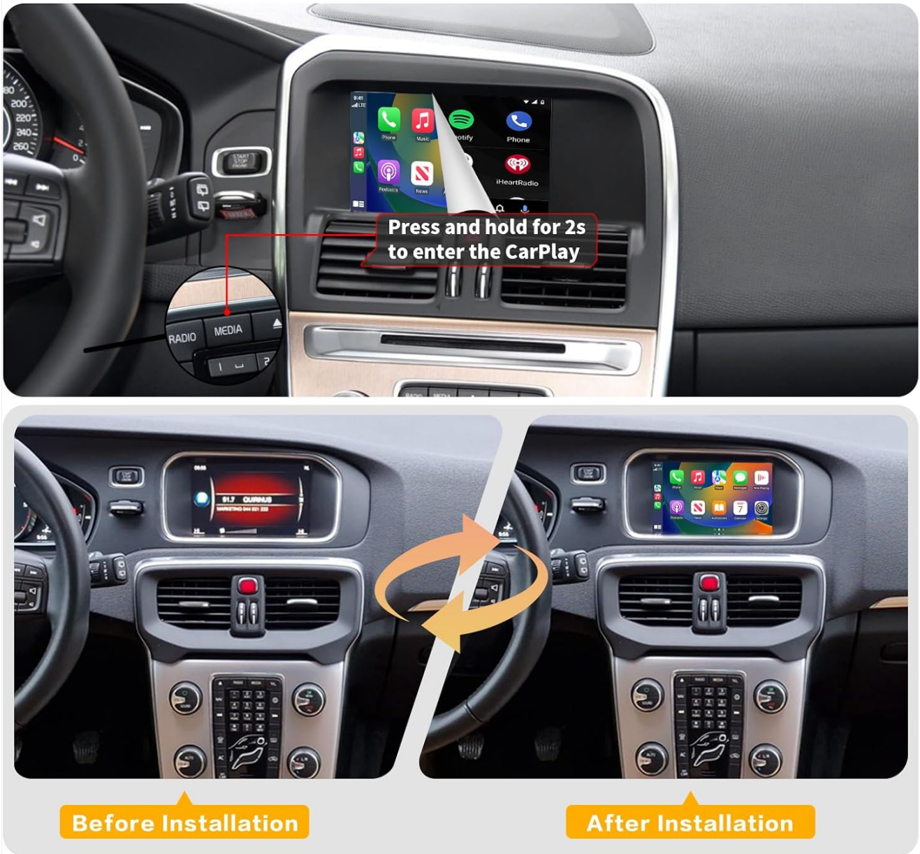
Image 5.1: How to switch between the original car system and the Carplay/Android Auto interface.
