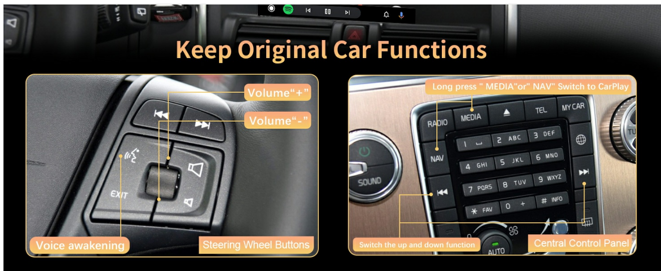
Image 5.7: How original car controls integrate with the new system.
