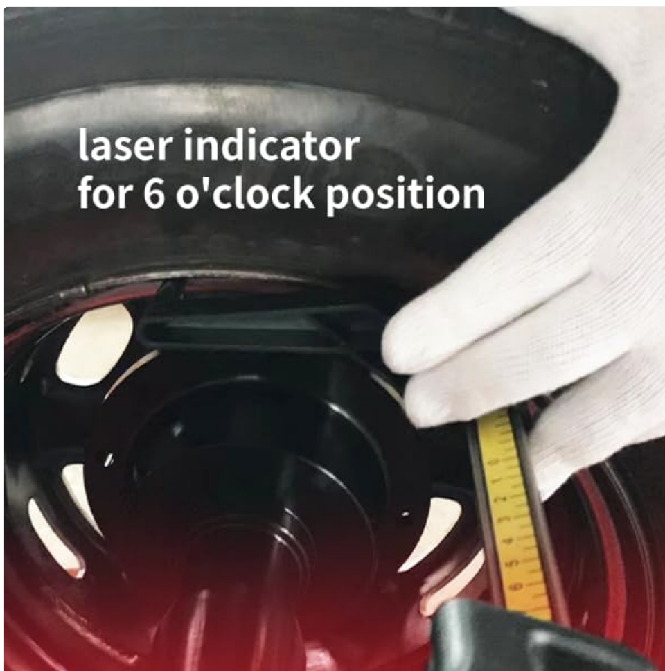
Figure 4: Laser indicator for precise weight placement at the 6 o'clock position.
