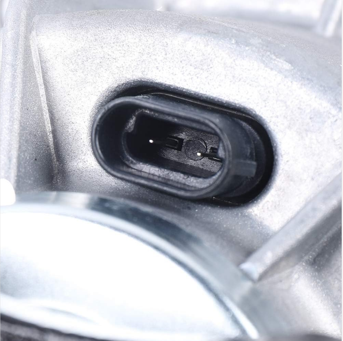
Image 2.1: Close-up view of the electrical connector on the differential coupling assembly. This connector facilitates communication and power supply for the electronic clutch mechanism.
