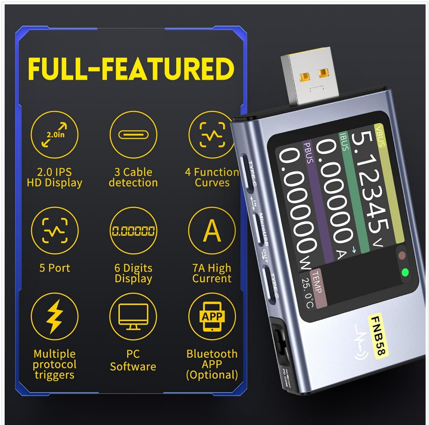
Figure 3.2: Key features displayed on the FNB58 USB Tester screen.
