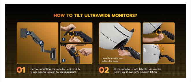
This diagram illustrates the steps for adjusting gas spring tension and loosening the tilt screw to ensure proper monitor movement.
