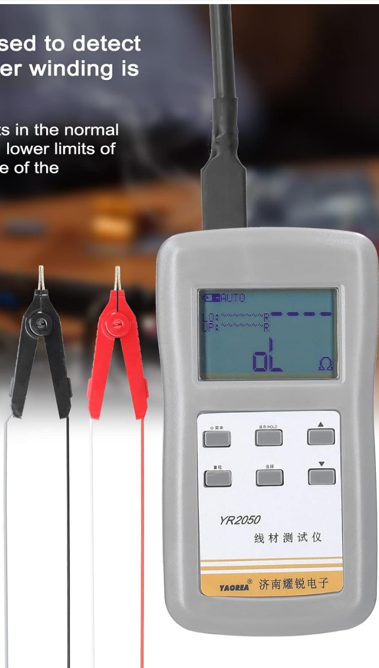
Figure 6.2: The YR2050 being used to test transformer winding qualification. The meter allows setting upper and lower resistance limits for comparison.
