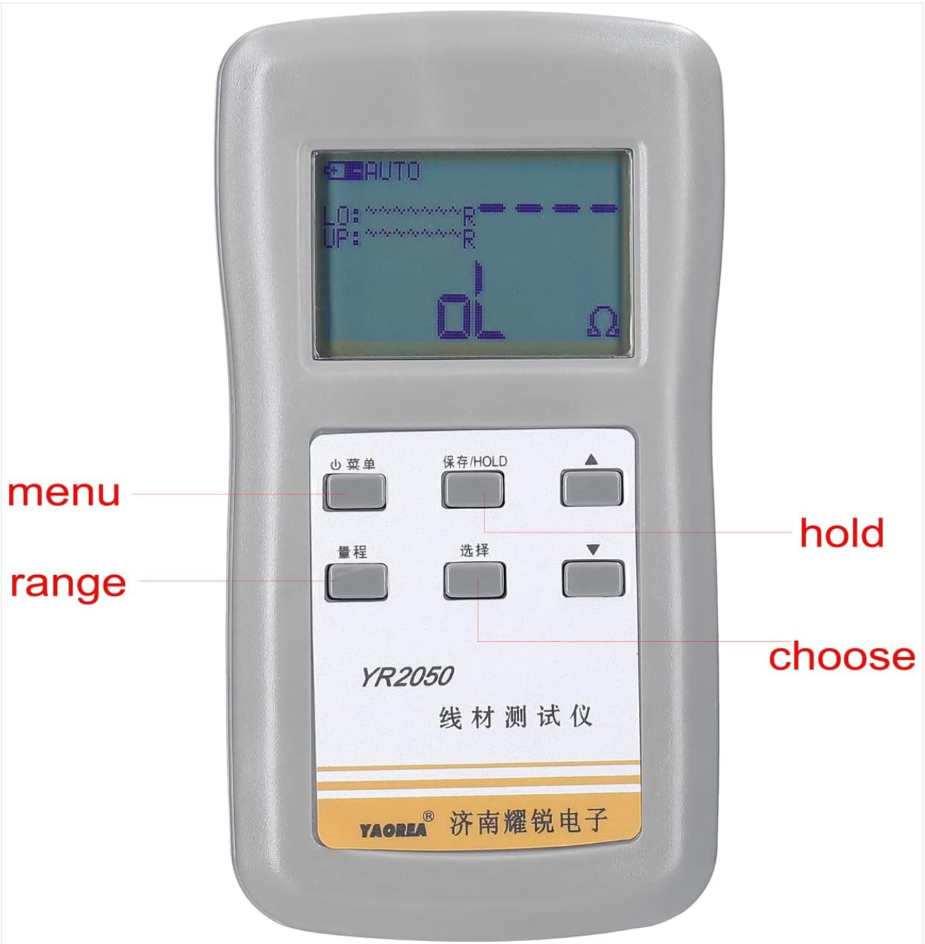
Figure 6.3: The YR2050's high accuracy is beneficial for measuring the resistance of precision current-sense resistors.
