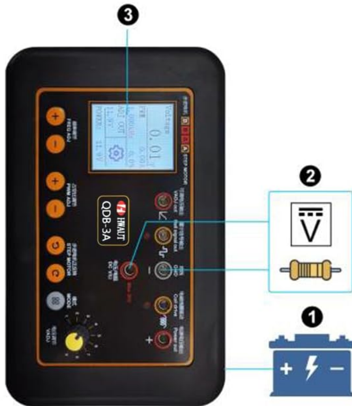
Figure 6.3: Connection diagram for resistance and voltage measurement.
