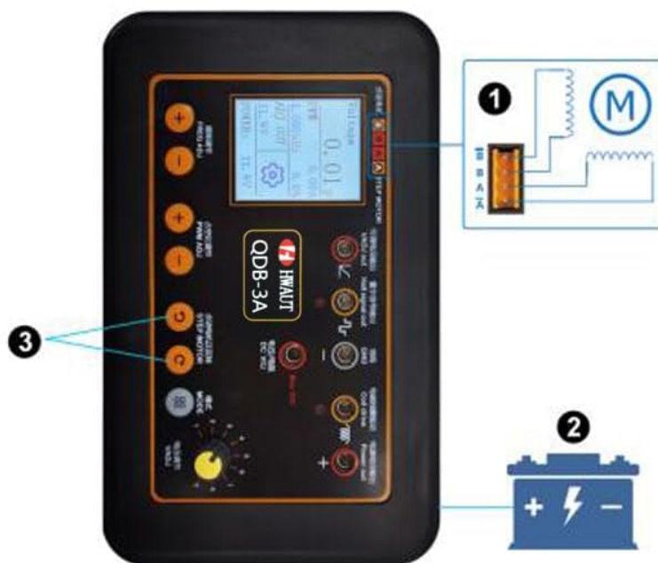
Figure 6.2: Connection diagram for step motor testing.
