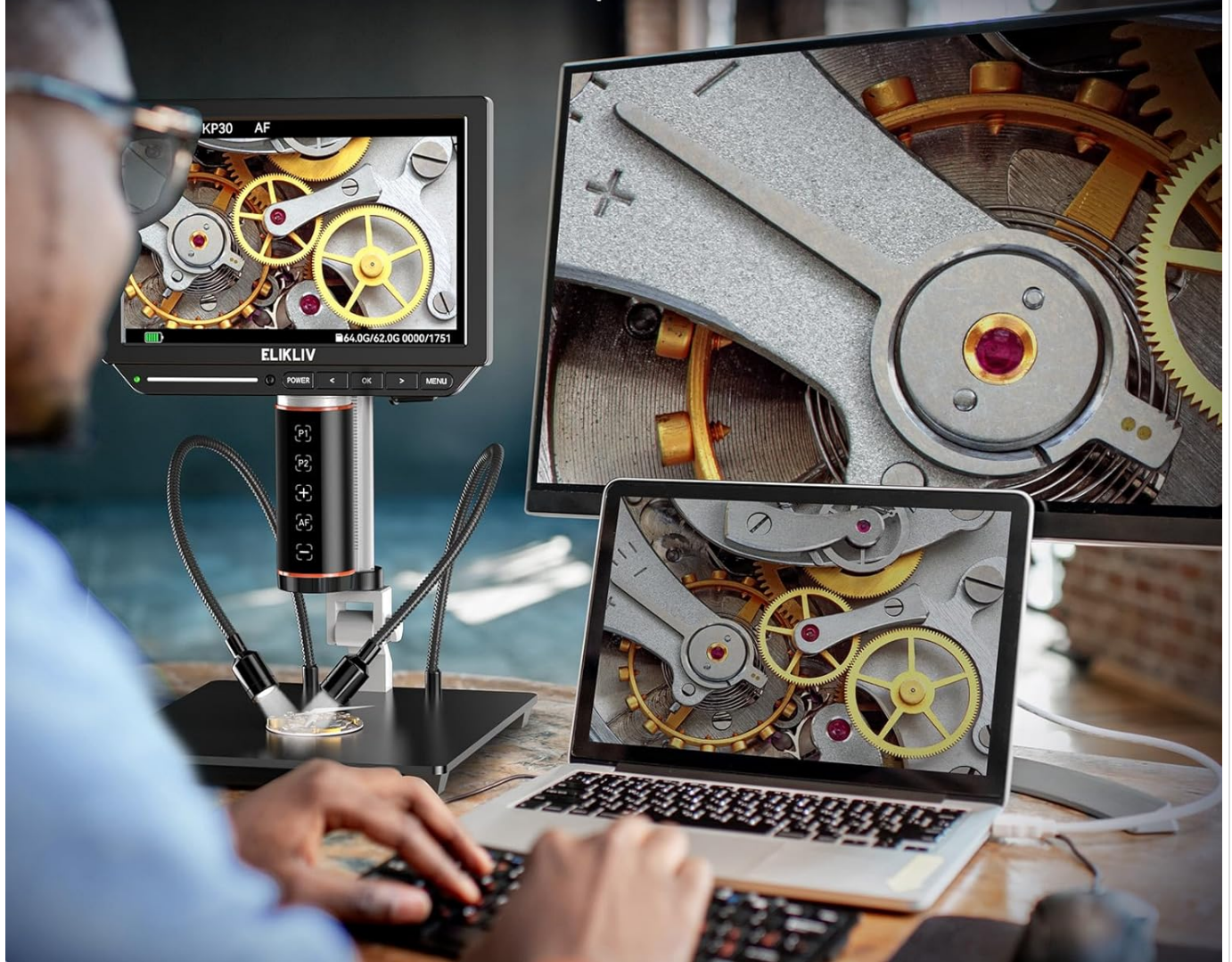
Image 6.4: The microscope displaying its feed simultaneously on its built-in screen, an external monitor, and a laptop via HDMI and USB.
