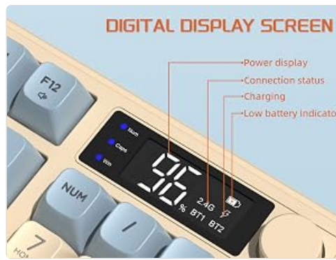
Image 4.1: Close-up of the M96 keyboard's LED display screen, showing indicators for battery level, connection status, Caps Lock, Num Lock, and Win/Mac mode.
