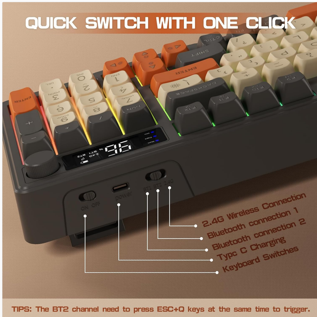
Image 4.3: Side view of the ZIYOU LANG M96 keyboard, indicating the power switch, 2.4G/Bluetooth mode switch, and Type-C charging port.
