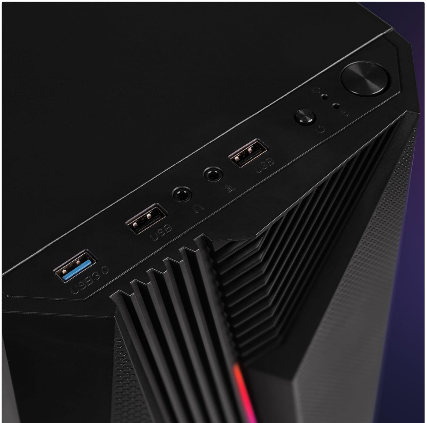
Figure 2.2: Front panel connectivity of the VIBOX I-100 PC, showing USB 3.0, USB 2.0, microphone, headphone jacks, RGB lighting control, and power button.
