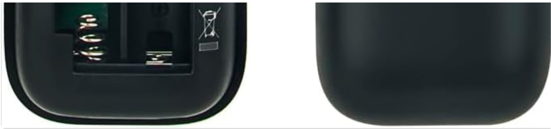
Figure 2: View of the battery compartment with the cover removed, showing slots for two AAA batteries.
