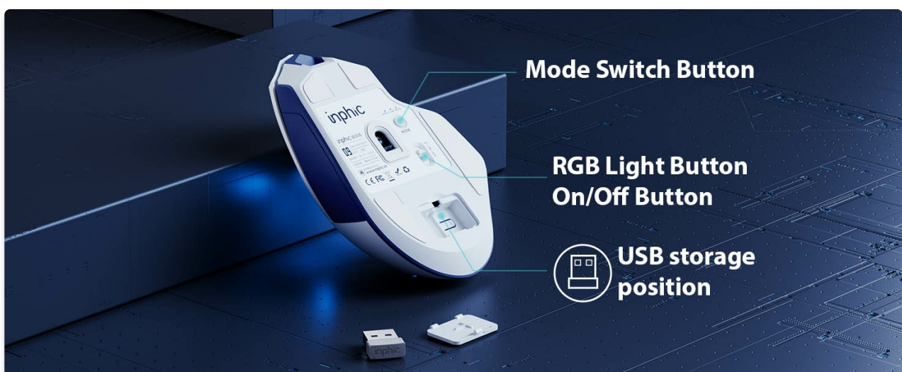
Bottom view of the INPHIC IN9 mouse, highlighting the mode switch button, RGB light button, On/Off button, and USB receiver storage position.
