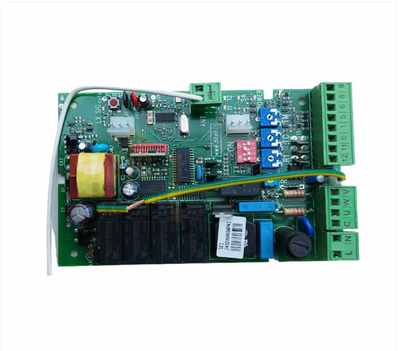
Figure 1: Ditec 61E1 230V Electronic Control Board. This image shows the main control board, typically used in gate automation systems.
