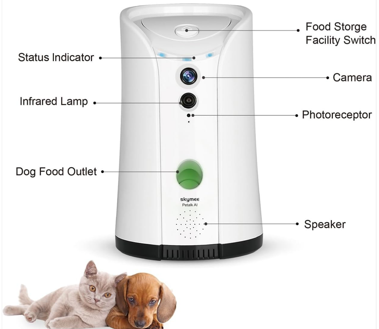
Image 1: Front view of the SKYMEE Petalk AI 5G, highlighting key components such as the Food Storage Facility Switch, Status Indicator, Camera, Infrared Lamp, Photoreceptor, Dog Food Outlet, and Speaker.
