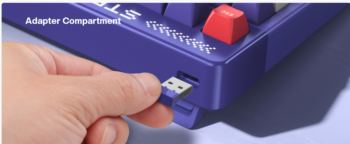
Image 3.3: Location of the 2.4GHz wireless receiver compartment.
