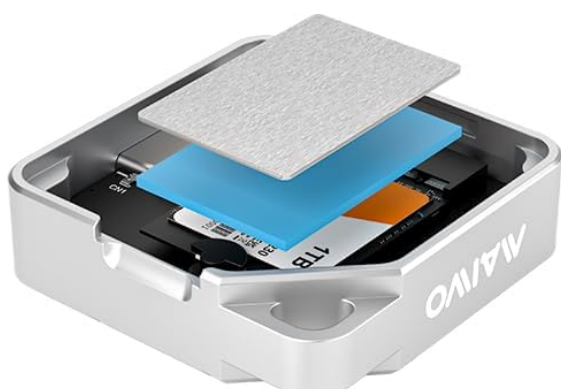
Figure 3: Visual guide for the tool-free SSD installation process.
