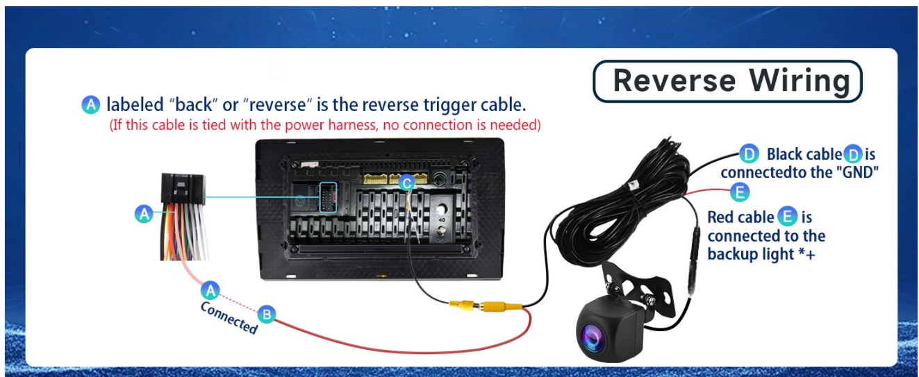
Image: A detailed diagram illustrating the connections for the reverse camera, including the video input, reverse trigger cable, and power/ground connections to the vehicle's reverse light.
