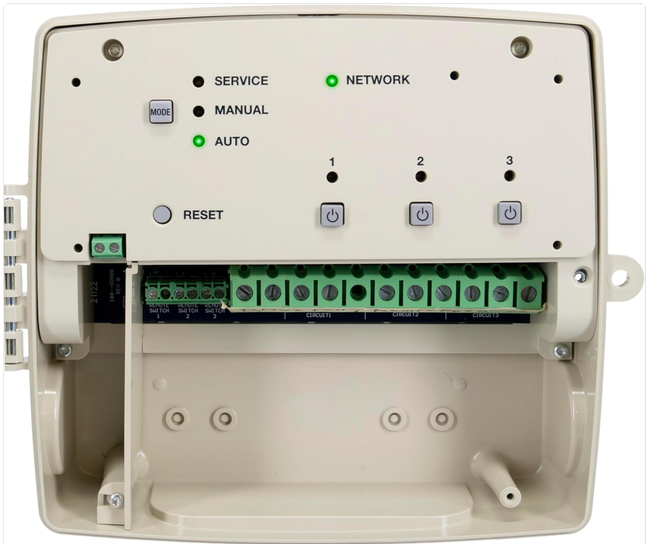
Figure 4.1: Internal View of PE733P Timer. This image displays the Intermatic PE733P timer with its front cover open. Visible are the internal control board with LED indicators for SERVICE, MANUAL, AUTO, and NETWORK status. Below these are the MODE and RESET buttons, along with three numbered manual override buttons for circuits 1, 2, and 3. The green terminal blocks for wiring input and three output circuits are clearly shown at the bottom of the control panel.
