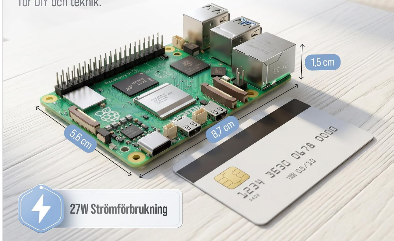
Figure 7: The compact size of the Raspberry Pi 5 board, with dimensions of 8.7 cm by 5.6 cm, shown next to a credit card for scale.
