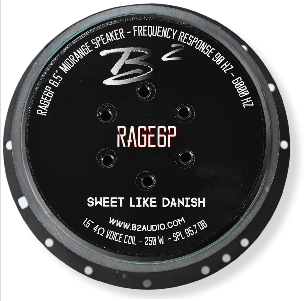
Image: The rear of the speaker displays key specifications and the B2 Audio branding, including the model number RAGE6P.
