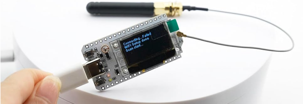
Image 2.1: Contents of the Wishiot ESP32 Lora V3 Development Board Kit, including the main board, antenna, and connectors.
