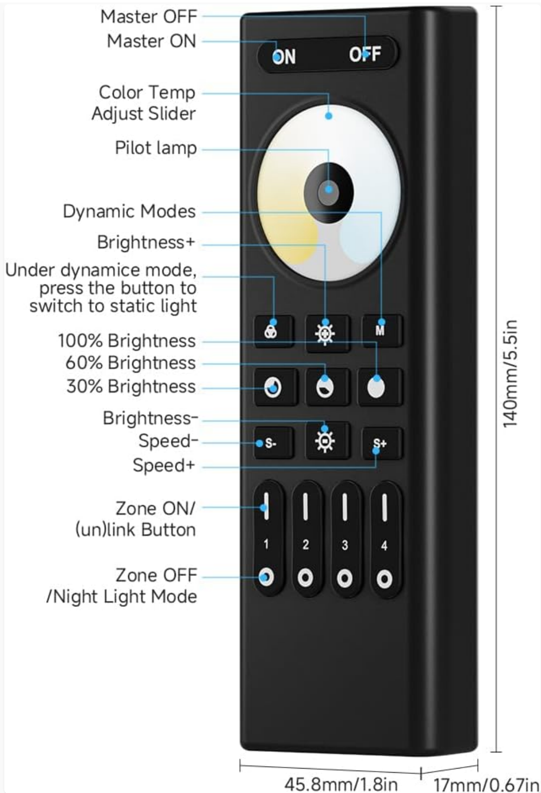
Image: A detailed diagram illustrating each button and feature on the FCOB CCT Remote RC02RFB, including ON/OFF, color temperature slider, brightness controls, dynamic modes, and zone selection.
