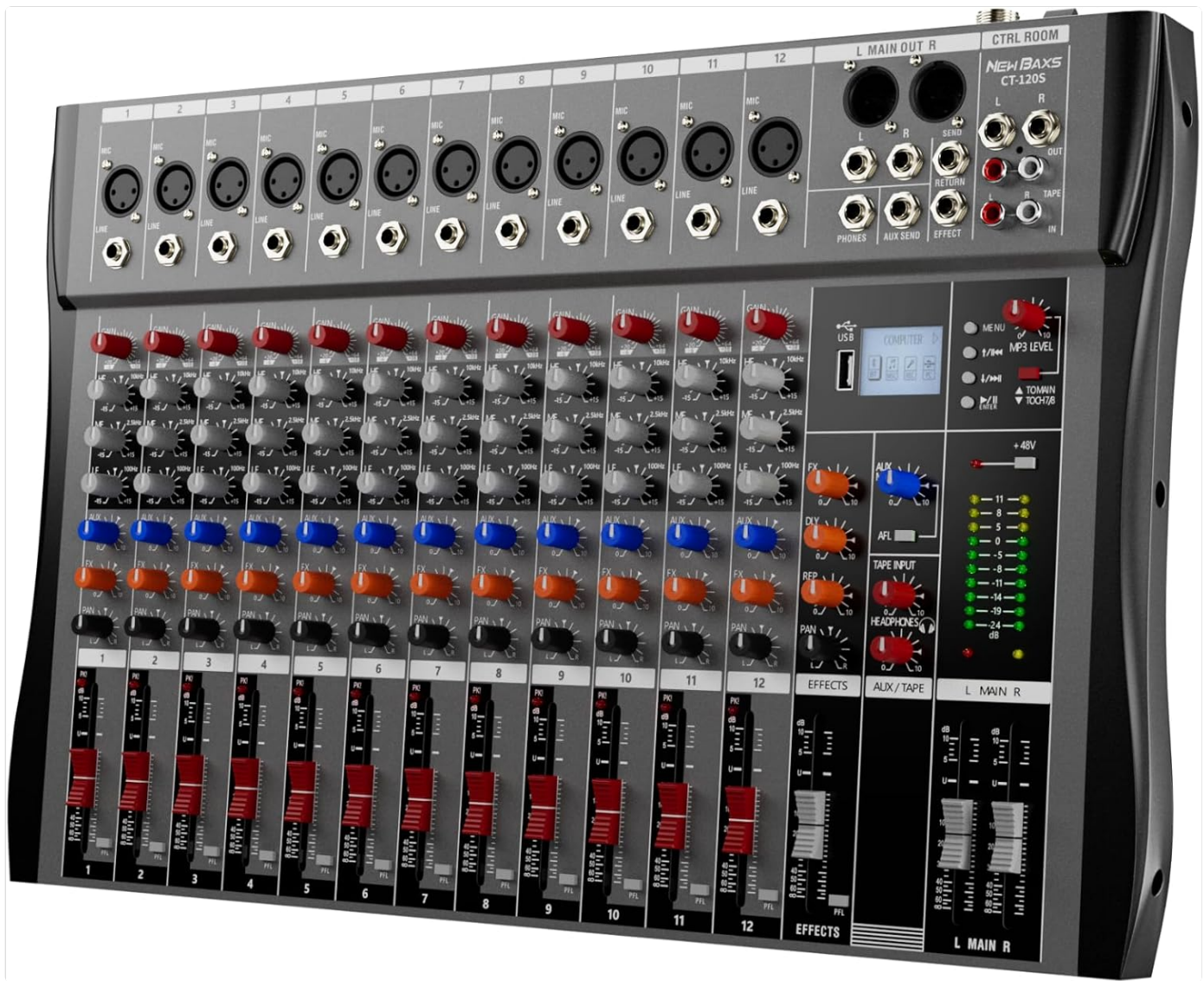
Figure 1: Main view of the NEW BAXS CT120S Professional DJ Audio Mixer.
