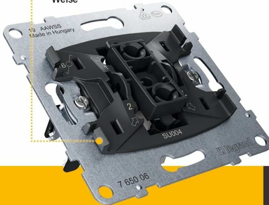
Figure 4.4: The 4-point spring system presses the frame firmly against the wall, facilitating a clean installation and compensating for uneven surfaces.
