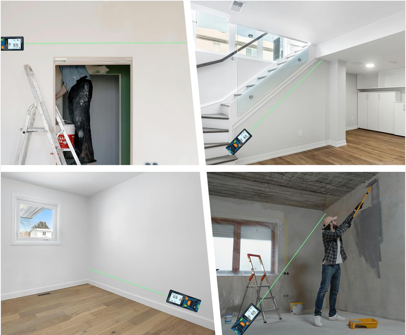
Image: An illustration depicting multiple measurement methods available on the device, including single measurement, continuous measurement, distance, area, volume, and Pythagorean calculations.
