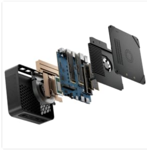
Figure 9: An internal view of the Mini PC, highlighting the accessible RAM and dual M.2 SSD slots for easy upgrades.
