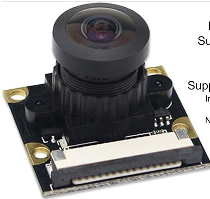
Image 1.1: Sanpyl Camera Module with OV5647 Sensor. This image highlights the main components of the camera module, including the OV5647 sensor chip and the adjustable lens.
