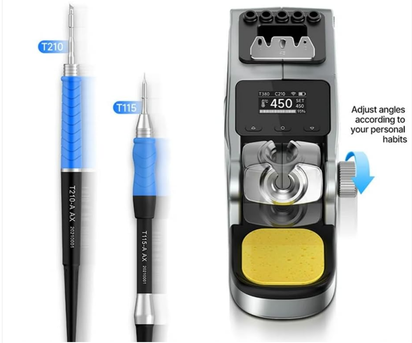
Figure 5.1: The T380 station demonstrating compatibility with T210 and T115 handles, and the adjustable sleep stand.
