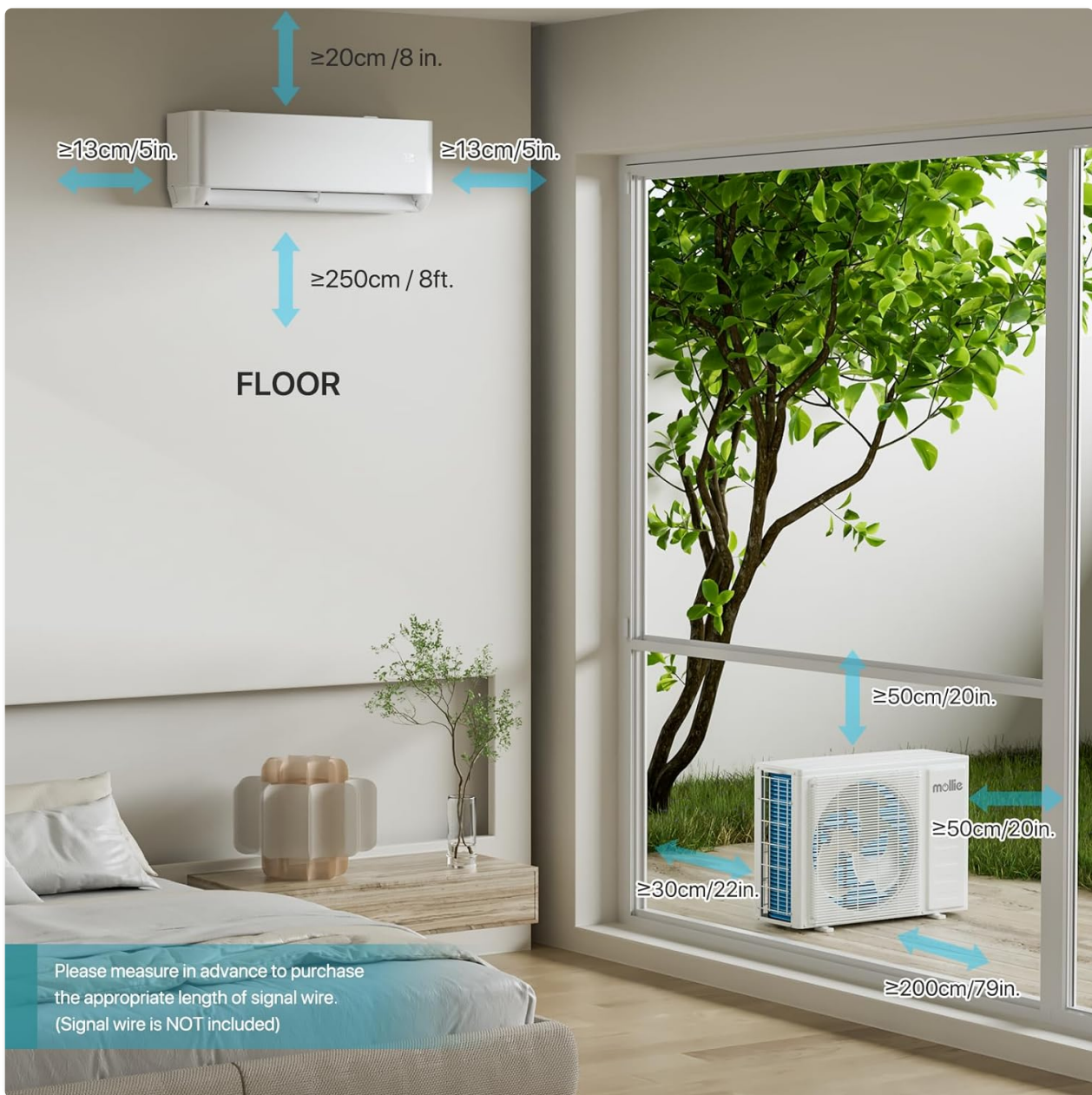
Figure 4.1: Recommended clearances for indoor and outdoor unit installation.
